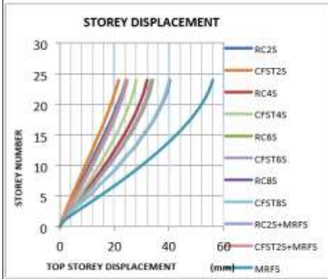
Fig.5 4 Storey displacement of the structure for the seismic loading for different diaphragm configuration
